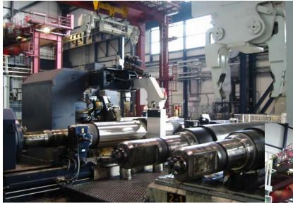
Cold Rolling Mill / Steel Coil Production Messurment Arm on Roll Grinding Mashine RACO Electric Actuator: Type T1N6
