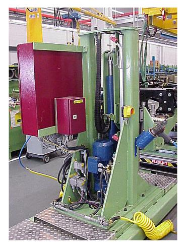
Automotive Machinery & Equipment Assembly Line Lift System
