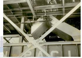
Unit train Loading Facility with SM2 Actuator
