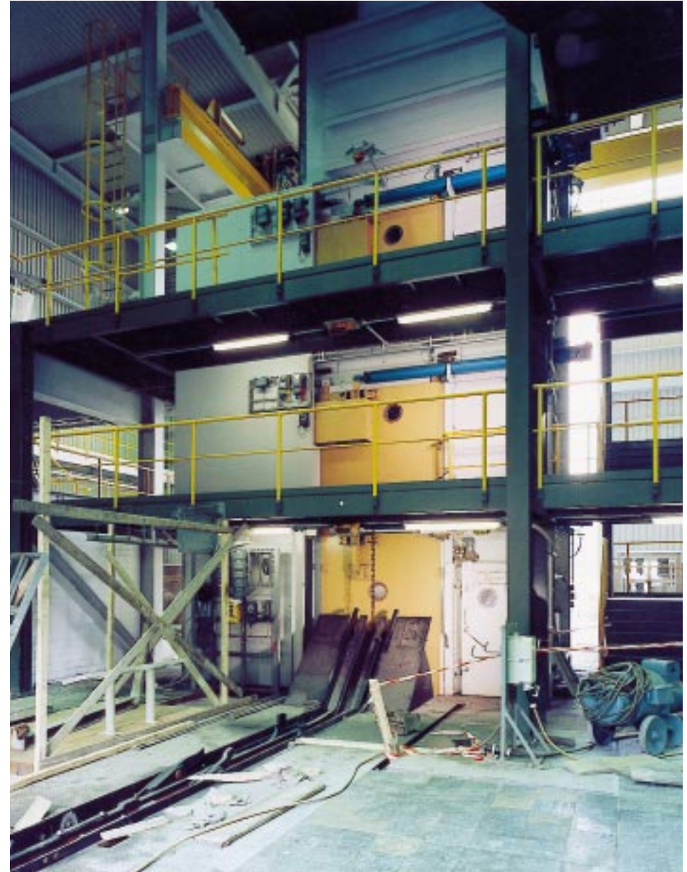
Mining elevator system with RACO rotary actuators type DM IV and RACO electric cylinders type T1K4 for locking, type M1F6 and type M1K7 for door operating.
