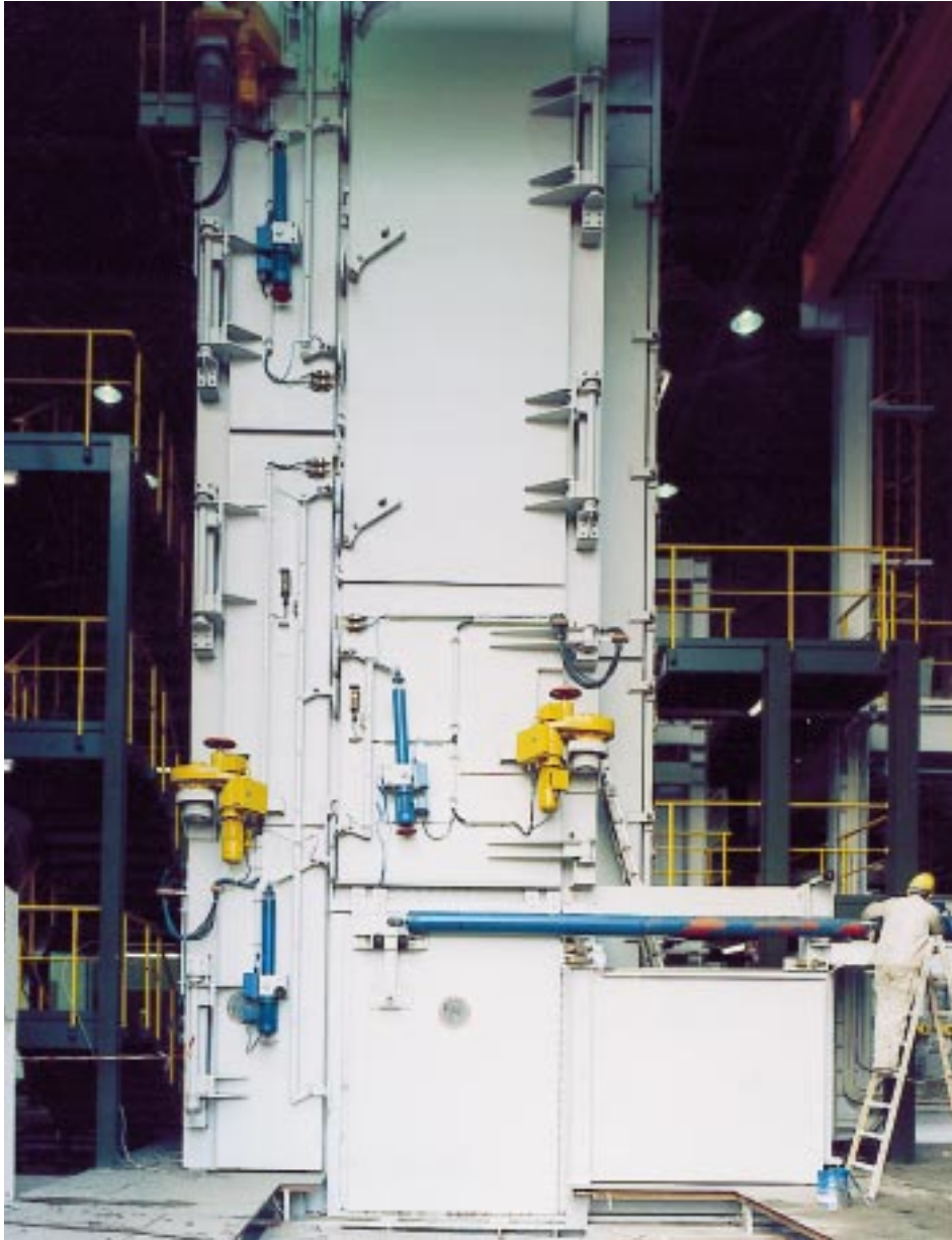
Mining elevator system with RACO rotary actuators type DM IV and RACO electric cylinders type T1K4 for locking, type M1F6 and type M1K7 for door operating.
