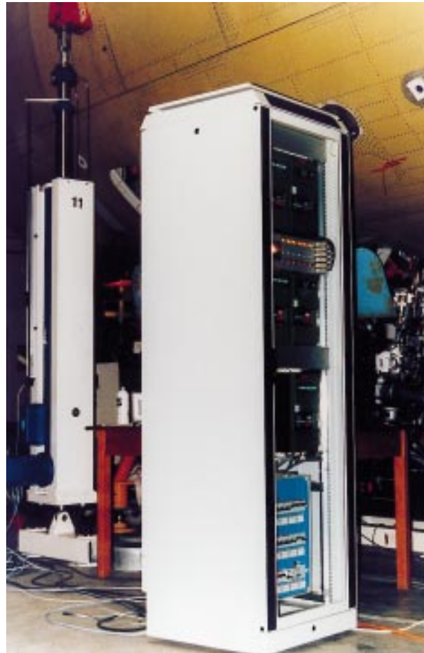
RACO electric cylinders type T1R7 40 kN, 800 mm
