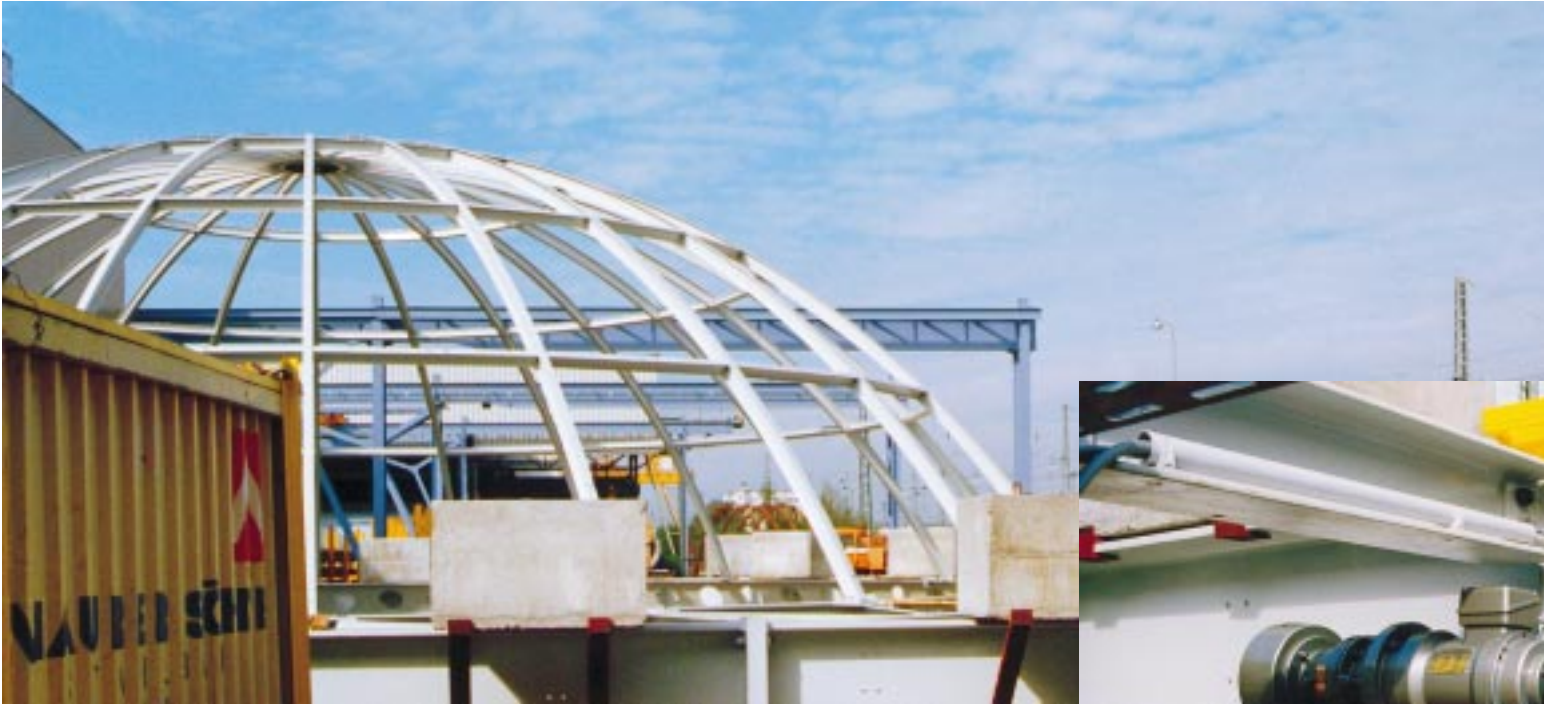
RACO electric cylinder type T1N7 30 kN thrust, 200 mm stroke
