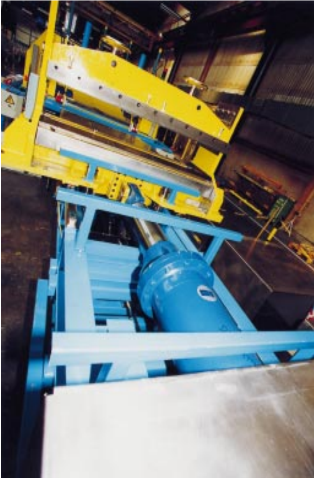
RACO electric cylinder type K1L10 300 kN thrust
